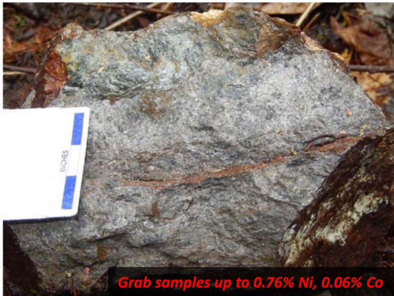
Ledgend massive pyrrhotite + pyrite ± pentlandite float
