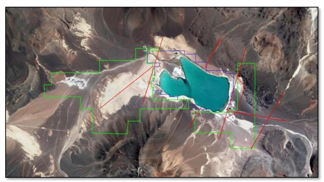
Figure 4. Laguna Verde Lithium Project land position showing the location of the pre-existing option property (blue outline) and the newly acquired Concessions (green outline). The location of geophysical gravity and TEM survey lines (red lines) are superimposed.
